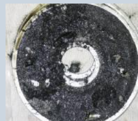
Upon changing to Addinol Ecogear 460M bypass filters were installed. Immediately after, the change particles were still clearly visible and had broken out of the tooth flanks
