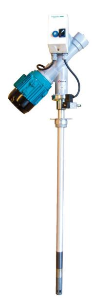
This high pressure 240V Electric grease piston pump is powered by an electric motor via a worm gear and is suitable for applications where compressed air is not available. The pump operates automatically by means of a pressure switch in the outlet, switching on or off the power according to the pressure limits set. (Please note that this function is only available if you have the control unit.)
