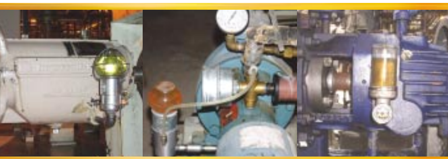
CLOSED SYSTEM OILER MOUNTED ON CENTER LINE OF DESIRED OIL LEVEL
