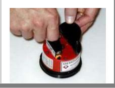
Carefully squeeze air out of the cartridge until grease begins to emerge from the outlet. This step avoids pump airlock and ensures an uninterrupted flow of grease to the piston pump.
