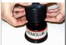
Place spring and compression plate into the transparent housing, with the compression plate facing the housing opening. Then place the housing assembly (transparent housing, spring and compression plate) over the lubricant cartridge which is seated on the red base. The compression plate should be seated evenly on the lubricant cartridge.
