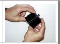
Place the cartridge on the pump inlet of the red housing. Make certain that the cartridge neck is well seated on the pump inlet.
