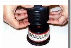
Lock the transparent housing in place with the black locking ring.
