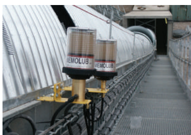
Mineral industry: lubrication of conveyor belt bearings.
