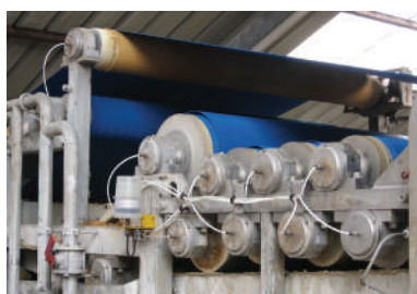
Food industry: lubrication of press ball bearings.
