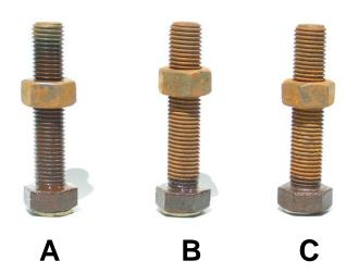
These three bolts were tested under the exact same conditions, all were placed in shallow containers so that the head was immersed in their respective product.
