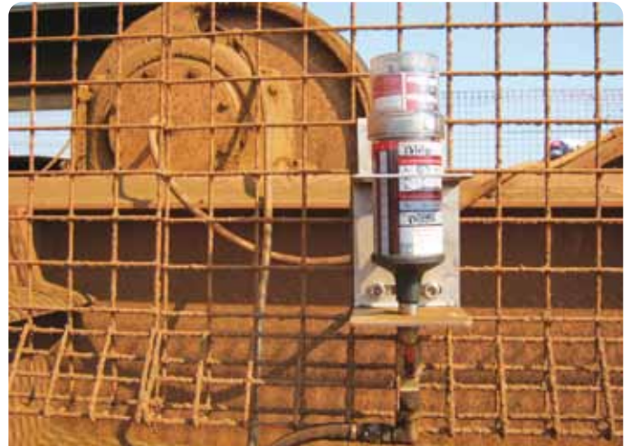
Application Seal purging with manual bearing lubrication Lubricator STAR VARIO L250 Install Kit K1CHC
