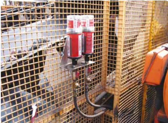
Application Bearing & seal Lubricator STAR VARIO L250 Install Kit K2CH
