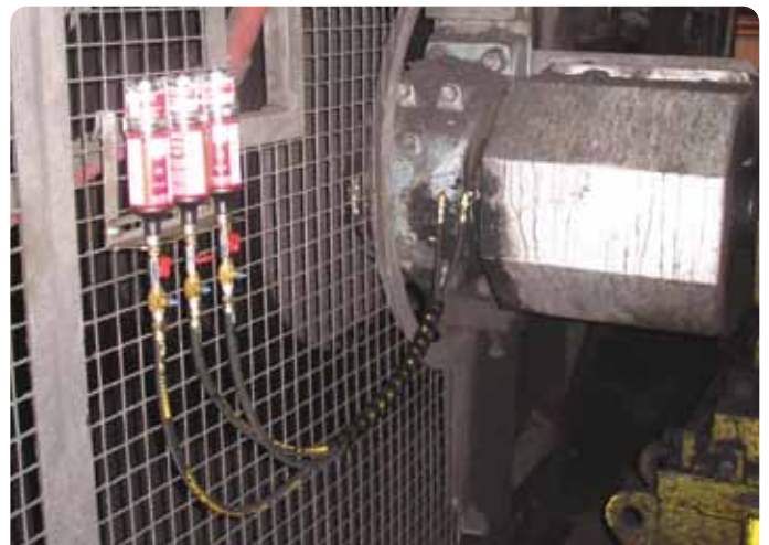
Application Bearing & seals Lubricator STAR VARIO L250 Install Kit K3CH
