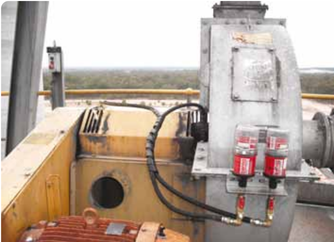
Application Jack shaft bearings Lubricator STAR VARIO M120 Install Kit K230
