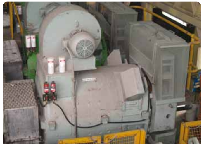
Application Dragline hoist motor Lubricator STAR VARIO M120 Install Kit Customised kit
