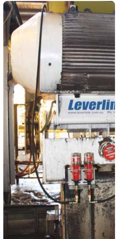
perma STAR VARIO remote mounted to an overhead electric motor.
