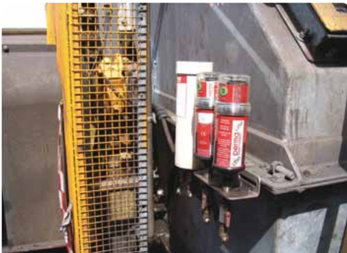
Application Bearing & seals Lubricator STAR VARIO L250 Install Kit K330
