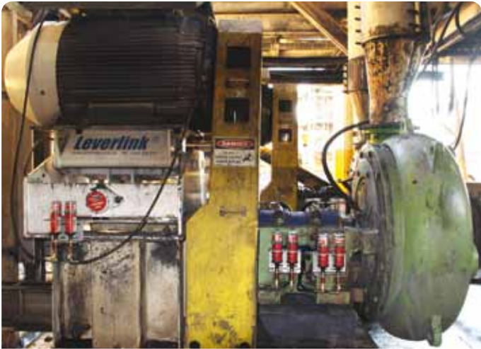
Application Krebs slurry pump Lubricator STAR VARIO L250 Install Kit K265C
