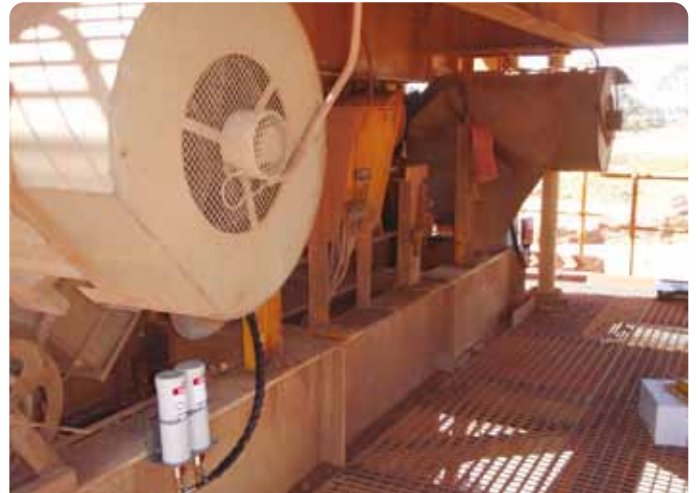
Application Motors driving scrubber Lubricator STAR VARIO L250 Install Kit K230C
