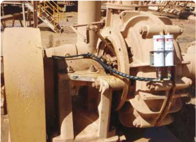
Application Warman slurry pump Lubricator STAR VARIO L250 Install Kit K265C
