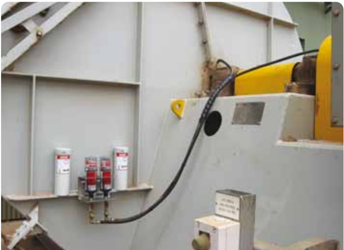
Application Jack shaft bearings Lubricator STAR VARIO L250 Install Kit K230C
