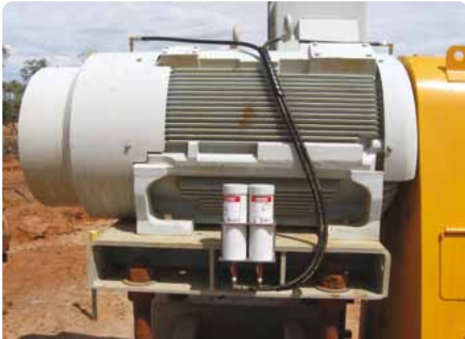
Application Motor driving Warman slurry pump Lubricator STAR VARIO L250 Install Kit K230C
