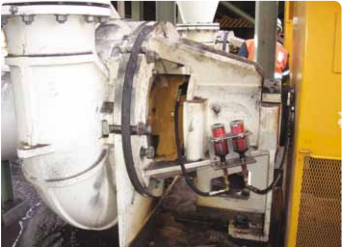
Application Metso slurry pump Lubricator STAR VARIO M120 Install Kit K230C
