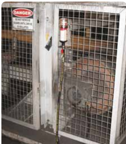
perma STAR VARIO remote mounted to a conveyor pulley bearing providing safe access for inspections and servicing.
