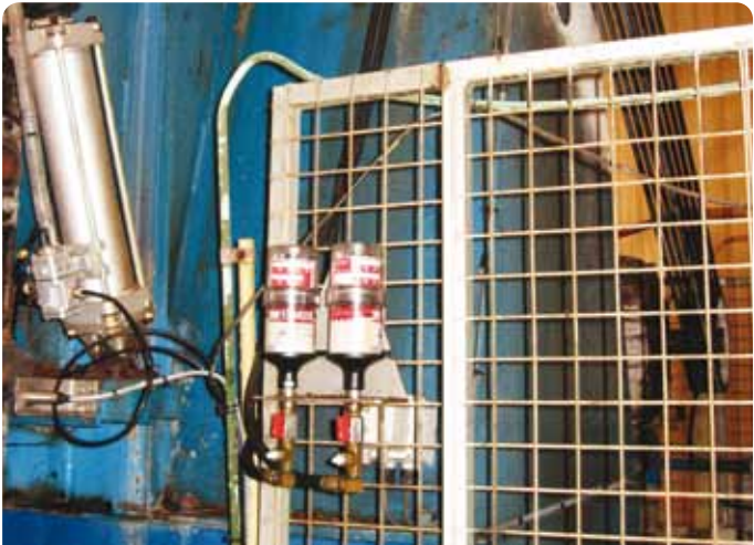
Application Jack shaft bearings Lubricator STAR VARIO M120 Install Kit K2CH
