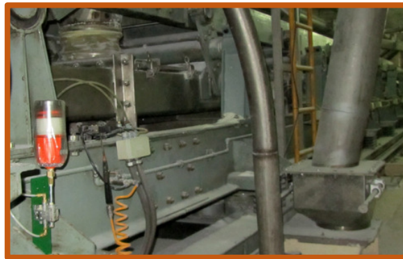
Conveyor bearings – 2 outlet divider valve and 250cc Pulsarlube Customer supply tube and fittings (Order Codes 91-GL250 & 41-LBK-2-000-O-BRA)
