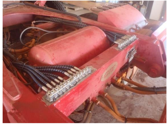
5 x 5 grease anchor blocks
