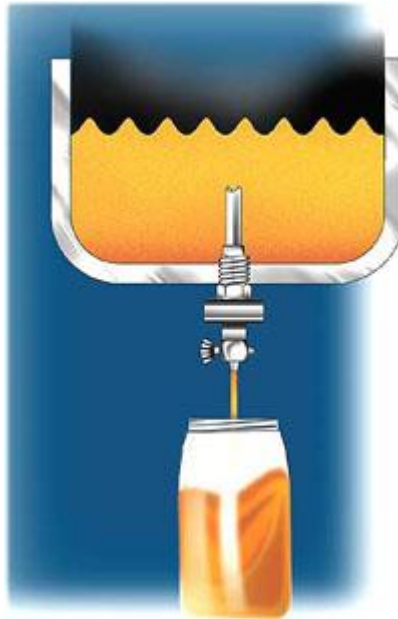
Figure 7. Drain Port Tap Sampling
