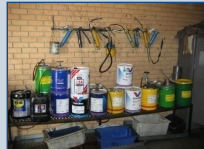
No documentation and unlabelled lubricants containers and grease guns.
