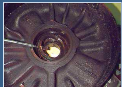
Shield was pressurised by excessive grease causing cage failure
